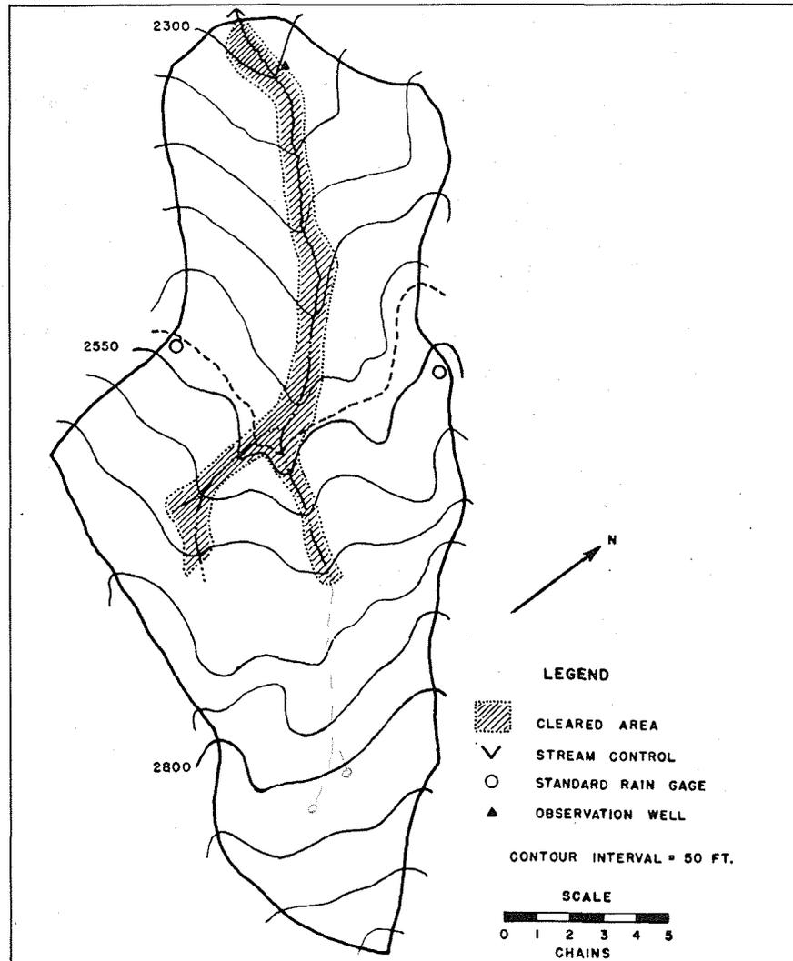
Fig. 1--Topographic map of Area Number 6, Coweeta Experimental Forest, showing area cleared of stream-bank vegetation
