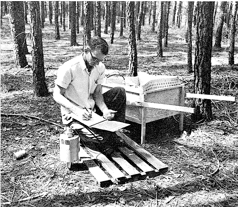
Figure 1.--Moisture content was determined with the Nuclear-Chicago Corporation P-19 Moisture Probe and Model 2800 Scaler. Spacing and relative size of the stand is shown in background.
