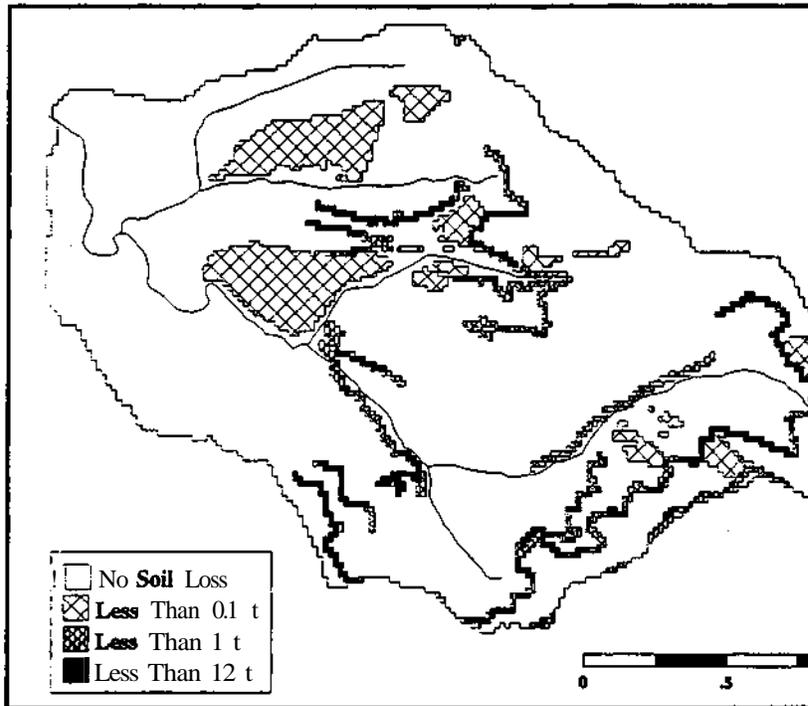
Figure 1. USLE Predicted Soil Erosion in a 1140 ha Watershed Given Poorly Roads and Average Annual Precipitation.
