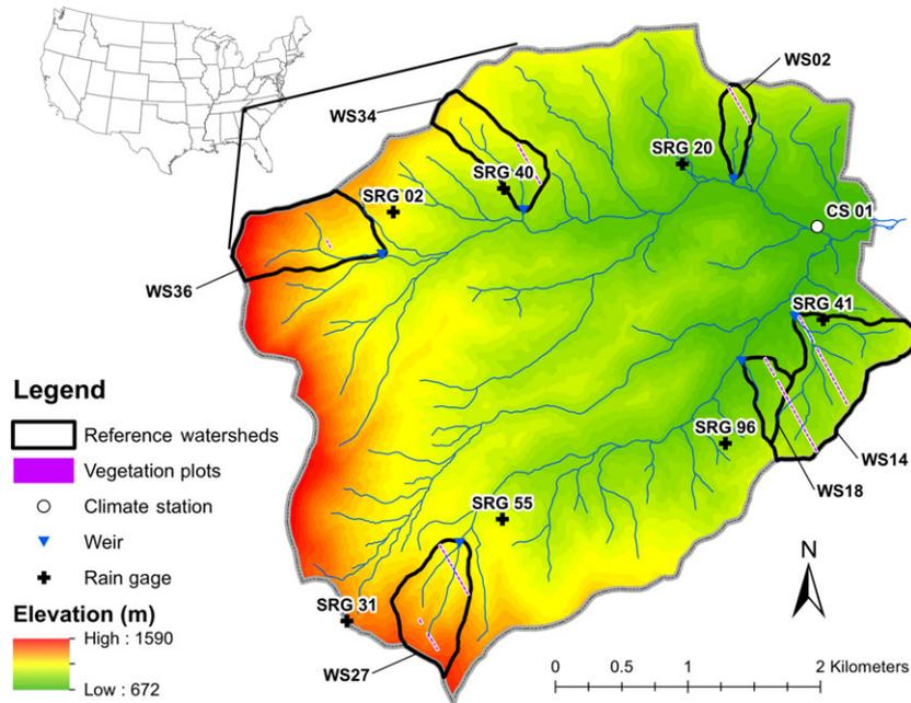
**Fig. 1** Site map of Coweeta Hydrologic Laboratory in Otto, NC showing reference watershed boundaries, vegetation survey plots, weirs, standard rain gauges (SRG), and long-term climate station (CS). Vegetation survey plots shown are only those in the reference watersheds that were sampled in 1934, 1970, 1990, and 2010.
