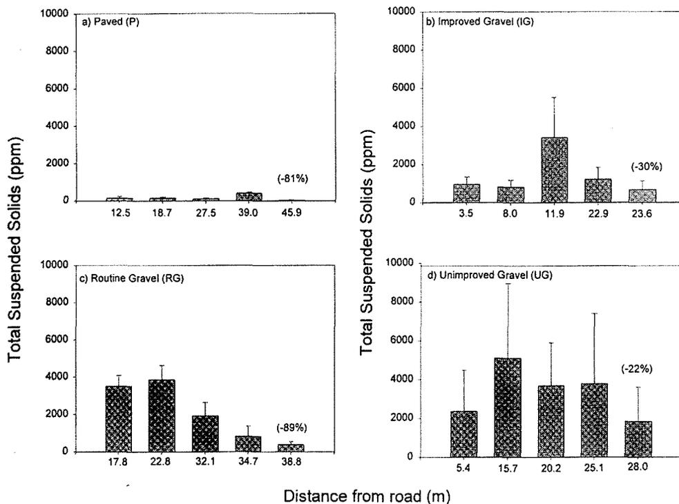
**Figure 2. Comparison of total suspended solids (TSS) along transects for each road surface type. TSS values and distances (m) are means for each collector location within a road surface type ( $n = 3$ ). Values in parentheses represent percent reduction in TSS from the closest to the farthest collector from the road. Error bars represent one standard error of the mean.**
