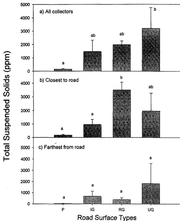
**Figure 1. Comparison of total suspended solids (TSS) movement among road types by (a) mean TSS for all collectors, (b) mean TSS for collectors closest to the road, and (c) mean TSS for collectors farthest from the road. Error bars represent one standard error of the mean. Means with the same letter are not significantly different.**
