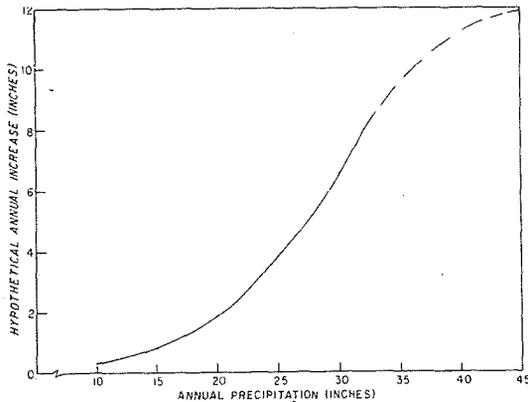
Figure 2. Yearly increase in streamflow in relation to annual precipitation for five watersheds in Arizona. The dashed line is an extrapolation of data from Hibbert et al. (1974).
