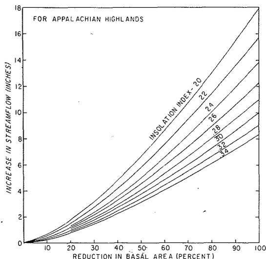
Figure 1. The first year increase in streamflow determined from the percent reduction in forest stand basal area and the insolation index (total langleys per year x 10<sup>-6</sup>) of the watershed.
