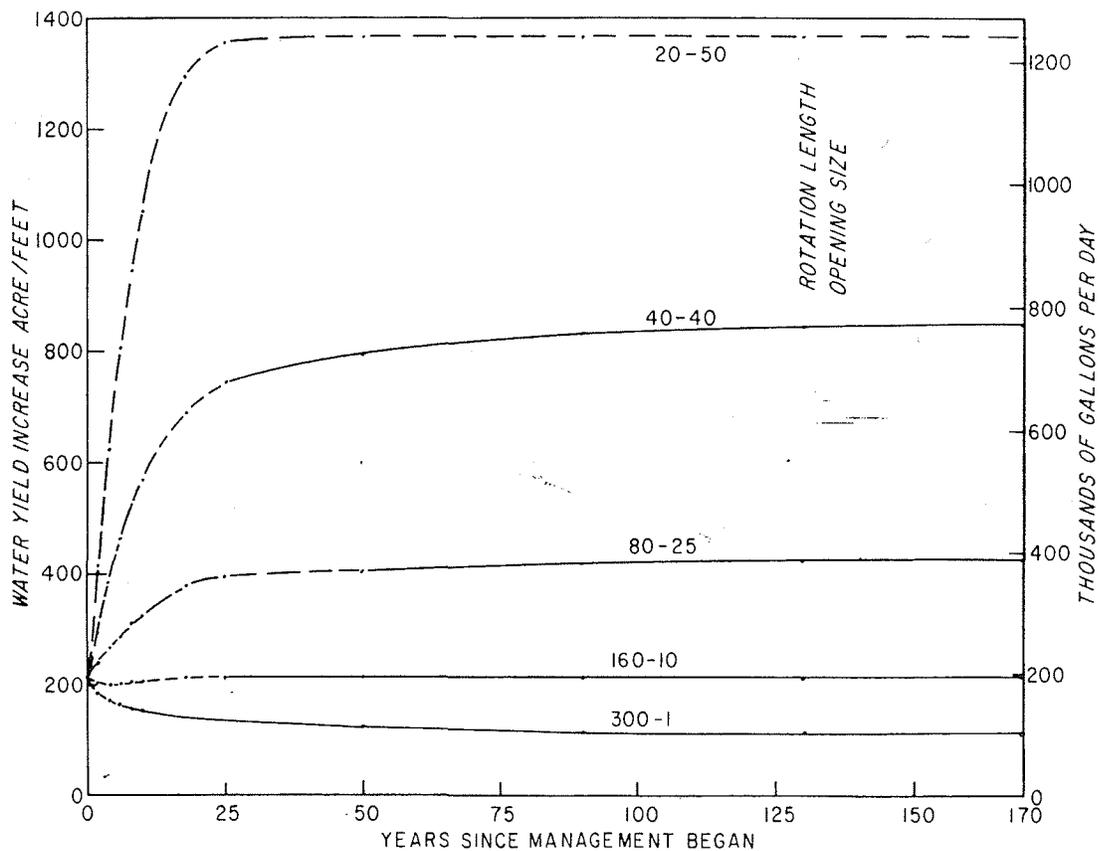
Figure 4. The increase in streamflow expected from managing the timber stand on a Southern Appalachian watershed under different rotation lengths in years and with different size openings. Each opening represents a clearcutting of the acreage specified.
