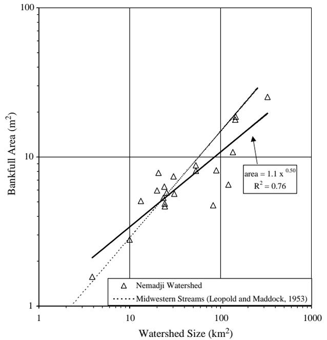
Fig. 4. Regional hydraulic geometry curve of bankfull channel area for study streams in the Nemadji watershed, Minnesota as compared to regional curves for Midwestern streams derived by [Leopold and Maddock \(1953\)](#).
