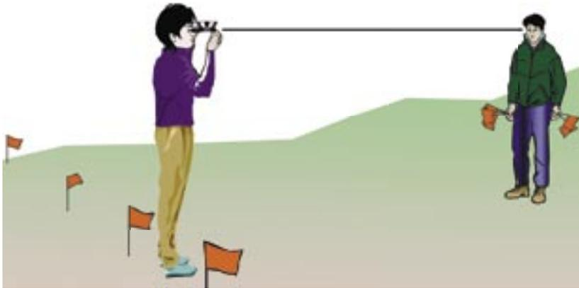
3. The flag person may mark the position (to be the centerline of the road) with plastic survey flags, wooden stakes, paint on trees or colored tape.
