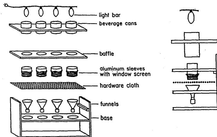
Fig. 2.6 A high-efficiency extractor for core samples of soil microarthropods. Soil cores contained in aluminum sleeves are inverted and heated from above with 5-watt lights. Fauna are collected in funnels below [Reprinted from Crossley and Blair, 1991. *Agric. Ecosys. Environ.* 34:187. Copyright with kind permission of Elsevier Science, Amsterdam, Netherlands].
