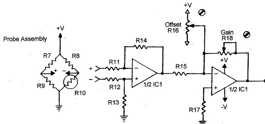
FIG. 3. Schematic diagram for the temperature amplifier. R7-R9—18 K  $\frac{1}{4}$  w 5% resistors; R10—thermistor 10 K @ 25°C (Radio Shack); R11-R14—10 K  $\frac{1}{4}$  w 5% resistors; R15—1 K  $\frac{1}{4}$  w 5% resistor; R16—5 K 10-turn PC potentiometer; R17—900 ohm  $\frac{1}{4}$  w 5% resistor; R18—5 K 10-turn PC potentiometer; IC1—TL072 dual FET operational amplifier.
