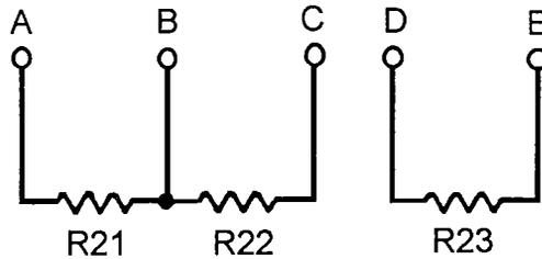
FIG. 5. Schematic diagram for the probe simulator. R21—59 K  $\frac{1}{4}$  w 5% resistor; R22, R23—2.7 K  $\frac{1}{4}$  w 5% resistor. Letters designate connector pins.
