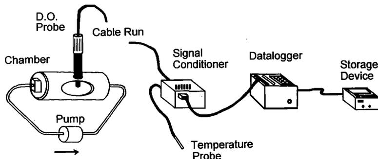
FIG. 1. Field apparatus for measuring dissolved oxygen uptake or release. The chamber, dissolved oxygen probe, and temperature probe are placed in the stream. The signal conditioner, datalogger, and storage device are on the bank.
