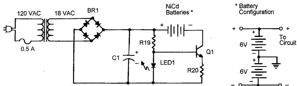
FIG. 4. Schematic diagram for the battery charger. R19—2 K  $\frac{1}{4}$  w 5% resistor; R20—5 ohm 5 w power resistor; C1—220  $\mu$ F 35 v electrolytic capacitor; BR1—5 amp bridge rectifier; LED1—light emitting diode; Q1—2N3055 NPN power transistor; miscellaneous—120 VAC-18 VAC 3-amp transformer, 1500-mAhr NiCd batteries, associated hardware.
