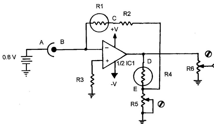
FIG. 2. Schematic diagram for the dissolved oxygen amplifier. R1—thermistor onboard YSI probe; R2—22 K  $\frac{1}{4}$  w 5% resistor; R3—3.3 K  $\frac{1}{4}$  w 5% resistor; R4—thermistor onboard YSI probe; R5—2 K  $\frac{1}{4}$  w 5% resistor; R6—10 K 10-turn precision potentiometer; IC1—TL072 dual FET operational amplifier. Letters designate YSI probe pins.
