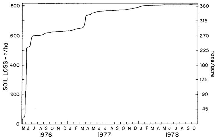
Figure 23.3. Cumulative soil loss from a forest road at a stream crossing in the first 2.5 ye after start of construction.
