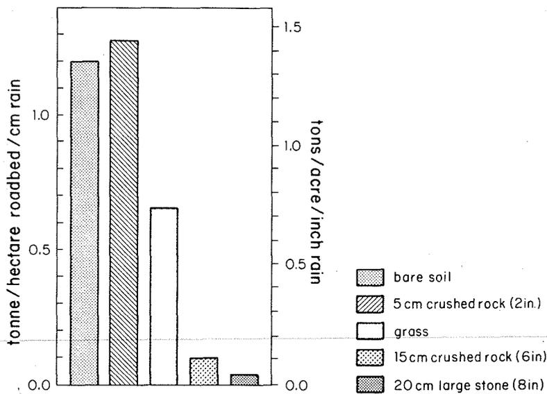
Figure 23.2. Soil loss rate for roadbeds with five surfacing treatments. Roads all constructed on sandy loam saprolite.
