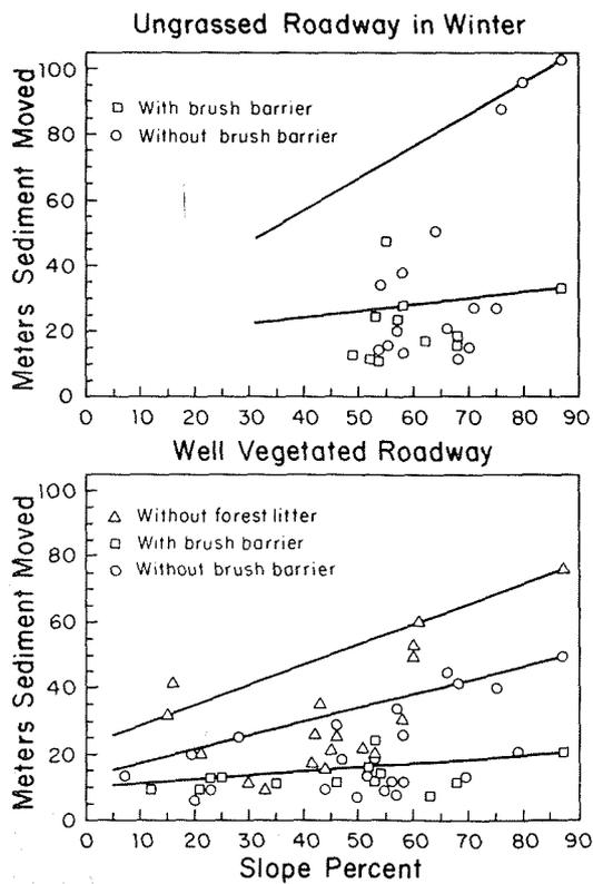
Figure 23.4. Lengths of sediment deposits downslope from roads are greatest where roadway is ungrassed by vegetation, and least where brush barriers and forest litter trap sediment flows.
