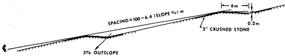
Figure 23.1. Diagram of the broadbased dip design for forest access roads.
