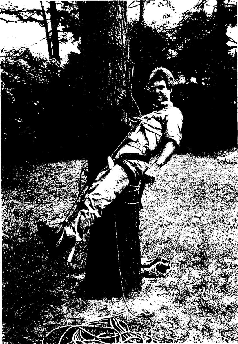
Fig. 2. — Assembled rope-climbing rig on author.
