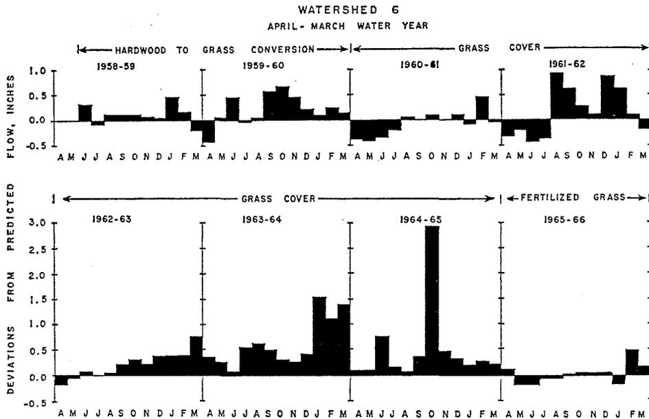
Fig. 2. Deviations of the monthly streamflow on watershed 6 from the predicted flow during the conversion from hardwood to grass and the six years under a grass cover.
