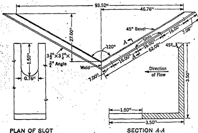
FIG. 1. 120-DEG V-NOTCH WEIR BLADE
