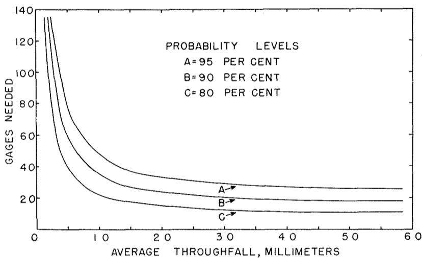
Fig. 2 — Cylindrical gages needed to sample throughfall in pine stands at 5 per cent accuracy and selected levels of probability.
