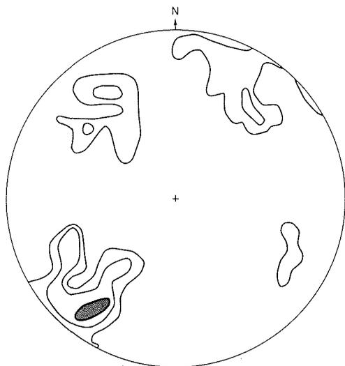
Figure 7.4. Bearing and plunge of 41 hinge lines. Contours 2.5, 5.0, 7.5% per 1% of net area.
