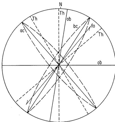
Figure 7.5. Generalized spatial relations between hinge-lines (*Fa*), tectonic joints (*bc*, and *ob*) and thalweg vectors (*Th*). Ec area projection.
