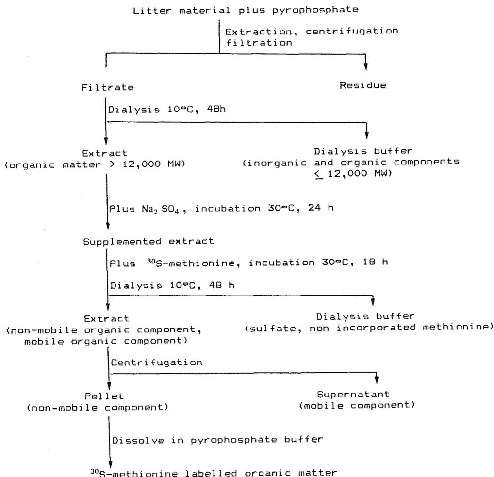
Fig. 1. Procedure for the preparation of  $^{35}\text{S}$ -methionine-labelled organic matter.
